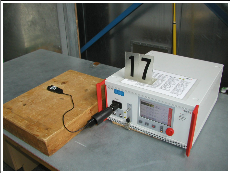
Figure 5 : Test Set-up "Immunity to fast transient disturbances (Bursts)"
