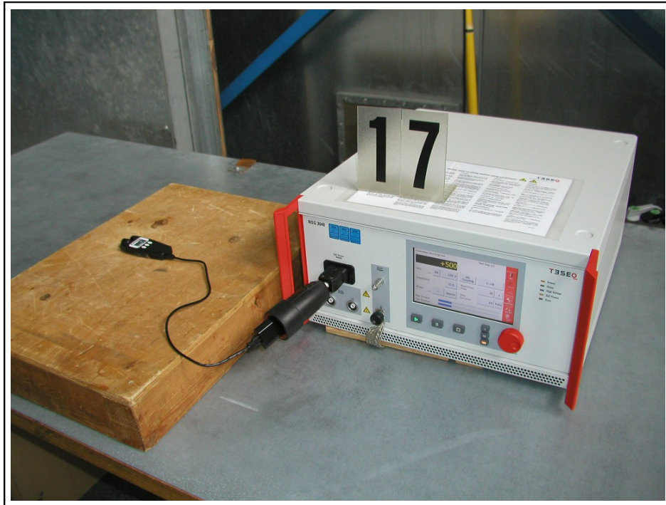
Figure 7 : Test Set-up "Immunity to surge pulses (Surge)"
